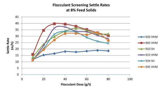
Figure 13-29: Lynx bulk tailings flocculant screening results
