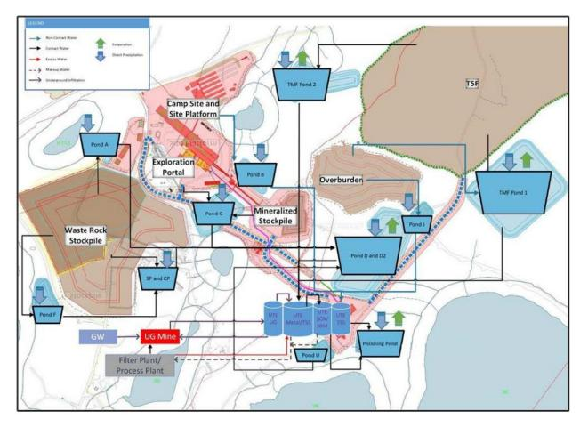
Figure 20-4: Water balance conceptual flow diagram – Phase 2
