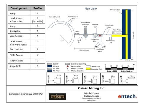
Figure 16-10: Typical level layout
