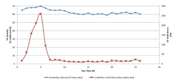
Figure 13-31: 190-mm pilot yield stress and underflow values produced during run time
