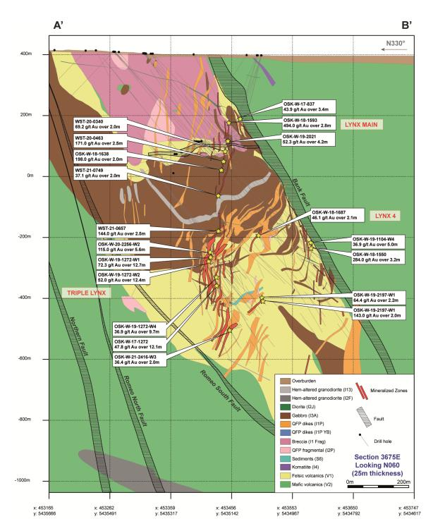
Figure 10-2: Representative geological cross-section showing the distribution of drill hole spacing and orientation in the Lynx area Significant assay results are also shown (Section 3675E). All lengths are core lengths ("CL") unless specified otherwise.
