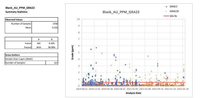
Figure 11-5: Time series plot for blank samples assayed by ALS (GRA22 Method) Failure limits set at 0.5 g/t Au (10x detection limit)
