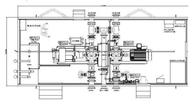
Figure 18-6: Fire water pump station layout
