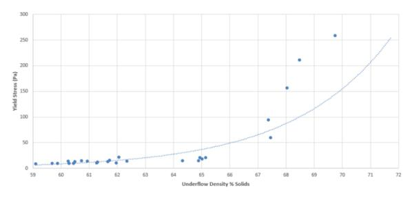
Figure 13-32: 190-mm pilot yield stress vs. underflow solids content
