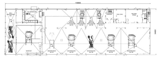
Figure 18-7: Truck shop layout (first floor)
