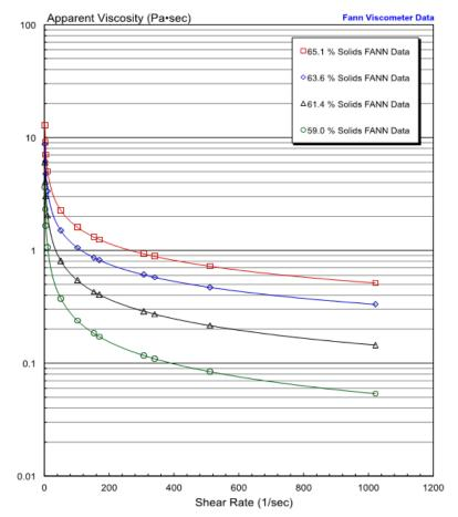
Figure 13-6: Apparent viscosity vs. shear rate
