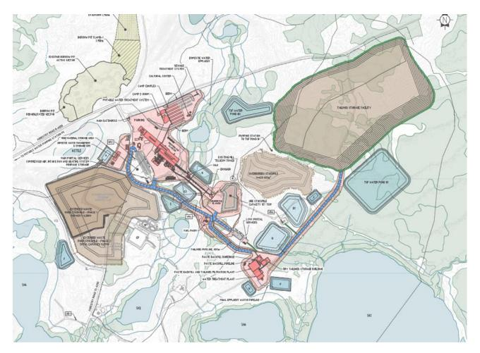
Figure 20-2: Surface water management infrastructures final layout – Windfall Mine Site
