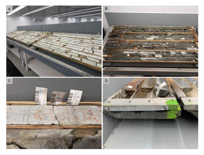
Figure 12-4: A) and B) Core review in the core logging facility, with C) Sample tags; and D) Identification tags
