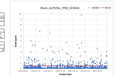
Figure 11-8: Time series plot for blank samples assayed by ALS (SCR24G Method) Failure limits set at 0.5 g/t Au (10x detection limit)
