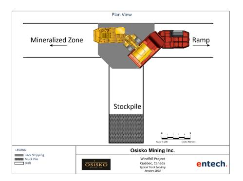
Figure 16-11: Typical level truck loading arrangement
