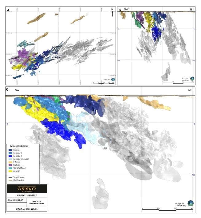
Figure 14-5: Main zone mineralized zones in the Windfall deposit A) Plan view; B) Cross-section view (looking northeast); and C) Longitudinal view (looking northwest)
