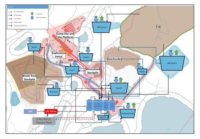
Figure 20-3: Water balance conceptual flow diagram – Phase 1
