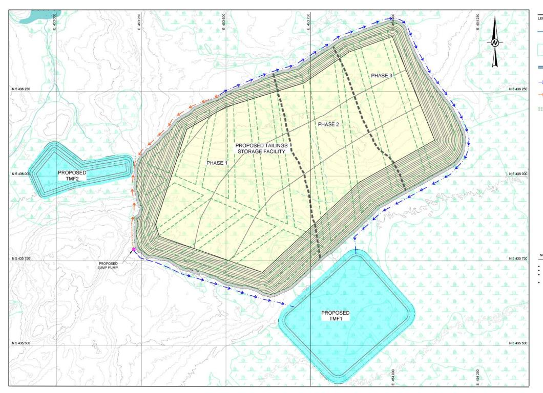
Figure 18-16: Plan view of the tailings management facility
