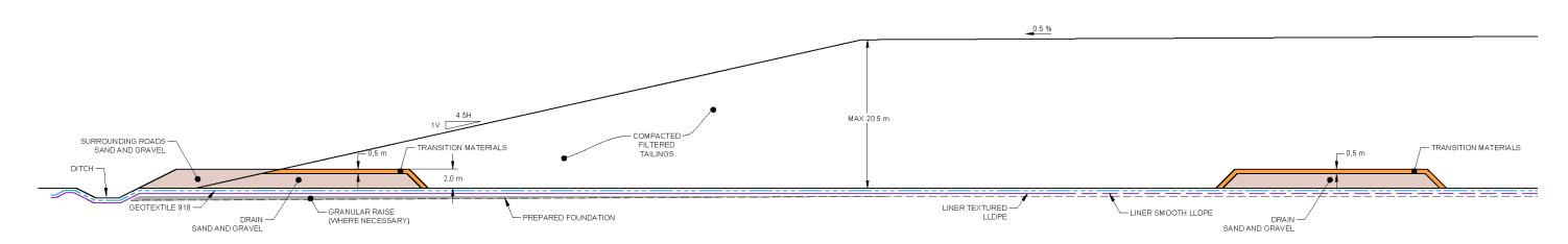
Figure 18-17: Typical cross-section of the tailings management facility
