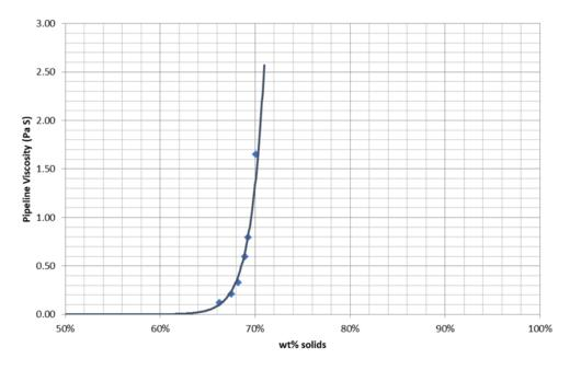
Figure 13-27: Pipeline viscosity vs. wt% solids
