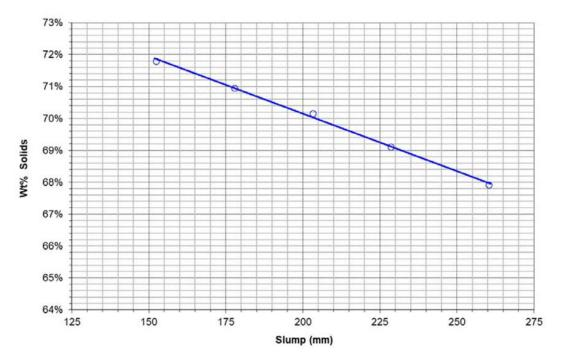
Figure 13-19: %Solids vs. slump for Tailings 37 µm sample
