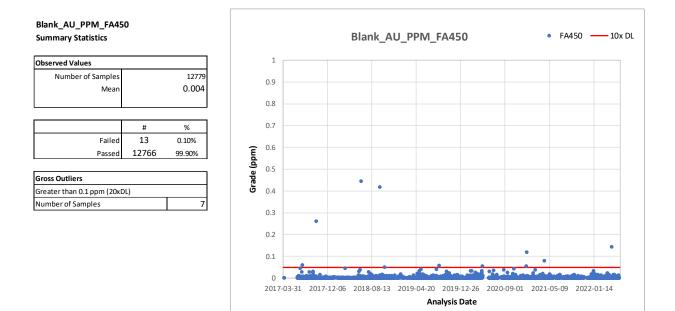
Figure 11-3: Time series plot for blank samples assayed by Bureau Veritas (FA450 Method) Failure limits set at 0.05 g/t Au (10x detection limit)
