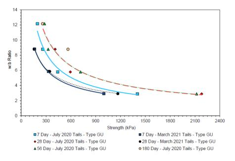
Figure 13-17: Water-to-binder ratio curves with "Type GU" binder
