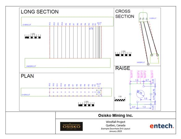
Figure 16-13: General arrangement for downhole stope design
