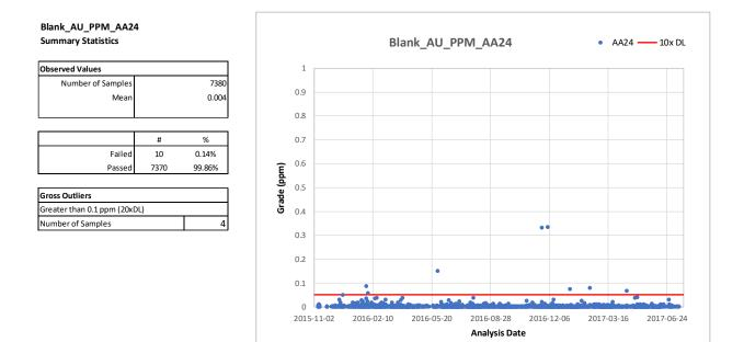
Figure 11-1: Time series plot for blank samples assayed by ALS (AA24 Method) Failure limits set at 0.05 g/t Au (10x detection limit)
