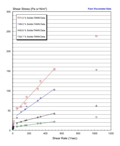
Figure 13-7: Shear stress vs. shear rate
