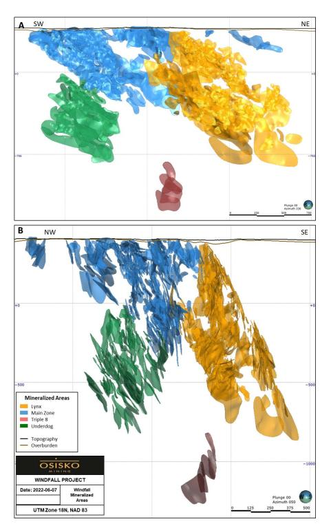
Figure 14-2: Mineralized domains modelled in the Windfall deposit A) Longitudinal view (looking northwest); and B) Cross-section view (looking northeast)
