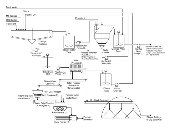
Figure 17-6: Tailings filtration plant simplified flowsheet
