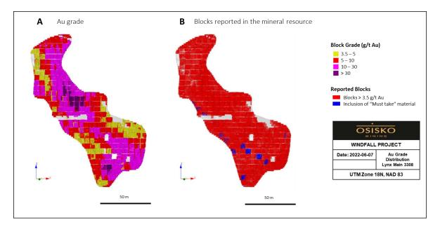
Figure 14-15: Example of blocks discarded or included in the mineral resource in lens 3308, Lynx Main zone A) Selection of blocks above 3.5 g/t Au; B) Reported blocks based on the mineable shape criteria
