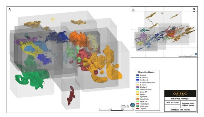
Figure 14-8: Bounding boxes of the block models A) 3D view; and B) Plan view
