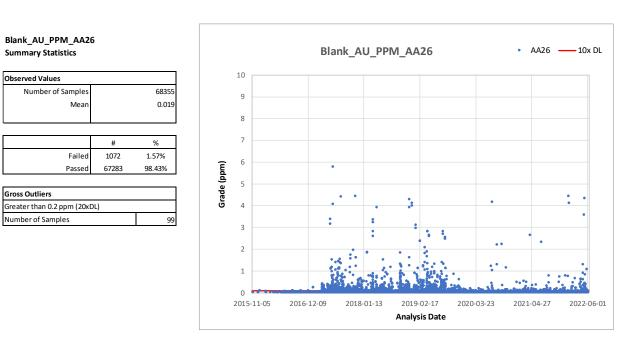
Figure 11-2: Time series plot for blank samples assayed by ALS (AA26 Method) Failure limits set at 0.1 g/t Au (10x detection limit)
