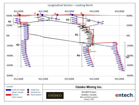
Figure 16-18: Primary mine ventilation system
