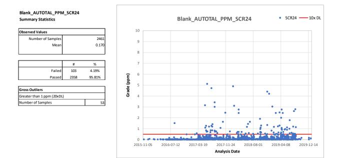
Figure 11-7: Time series plot for blank samples assayed by ALS (SCR24 Method) Failure limits set at 0.5 g/t Au (10x detection limit)
