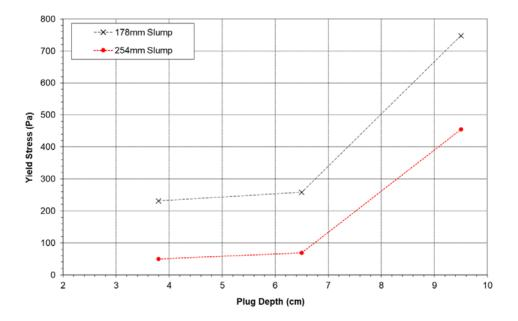
Figure 13-22: Plug yield stress for Tailings 37 µm sample
