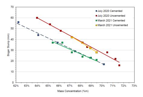
Figure 13-9: Boger slump vs. mass concentration
