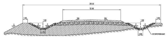
Figure 18-15: Haulage road – Typical cross-section
