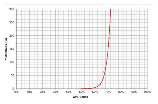
Figure 13-20: Static yield stress vs. %solids for Tailings 37 µm sample
