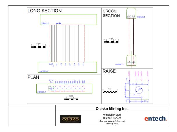
Figure 16-14: General arrangement for uphole stope design
