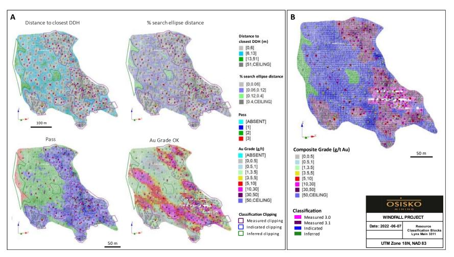
Figure 14-14: Example of resource classification for blocks in lens 3311 in Lynx Main zone A) Main criteria used for the decision-making in the drawing of the resource clipping boundaries; and B) Resource classification result
