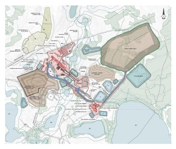
Figure 18-18: Surface water management infrastructure final layout - Windfall Mine Site
