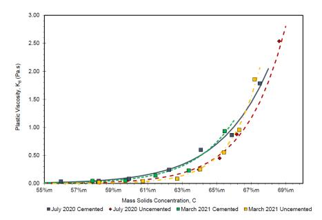
Figure 13-15: Plastic viscosity vs. mass solids concentration
