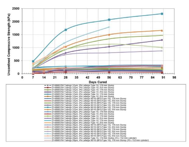
Figure 13-28: UCS results for samples Tailings 37 and 20  $\mu m$
