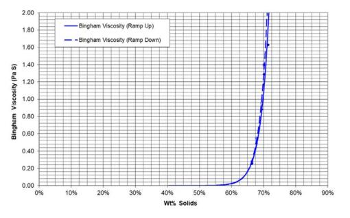
Figure 13-24: Bingham viscosity results for sample Tailings 37  $\mu m$  sample
