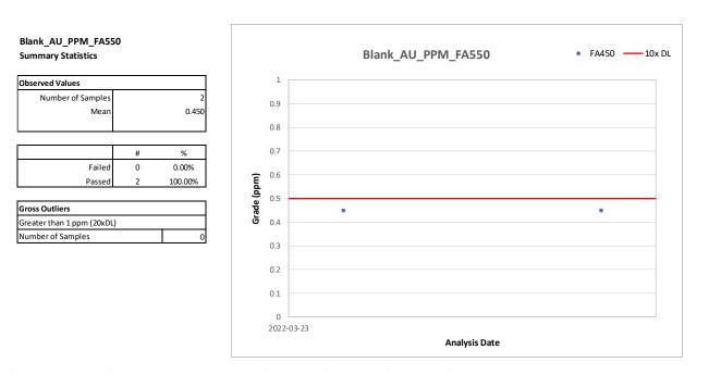
Figure 11-4: Time series plot for blank samples assayed by Bureau Veritas (FA550 Method) Failure limits set at 0.5 g/t Au (close to half detection limit of 0.9 g/t Au)
