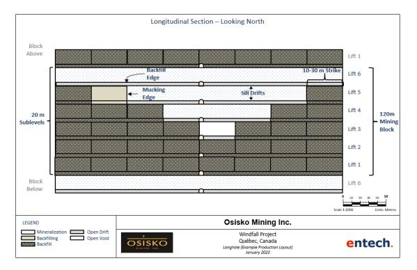
Figure 16-1: Production layout example
